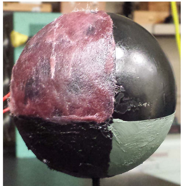
Fig. 3. Metal ball painted with Krylon flat black paint and three different makeup materials is shown. The following makeup paints have been applied to the ball: upper-left painted with gel makeup, lower-left painted with black makeup paint, lower-right painted with green makeup paint, and upper-right is makeup free.
